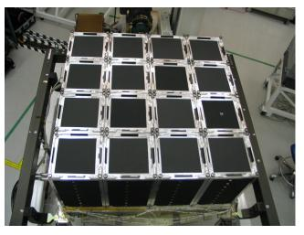
18 LAT TKR modules (16 + 2 spares) were integrated, tested and qualified for space use in 9 months
