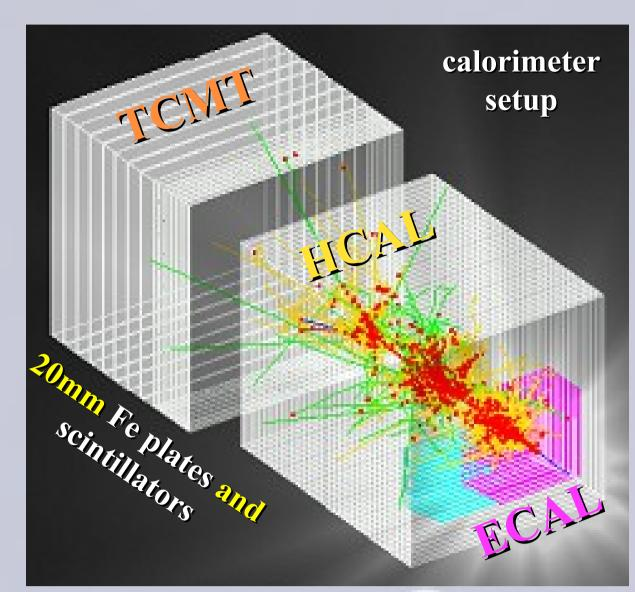
Prototype of calorimeters tested at accelerators of CERN and FERMILAB
