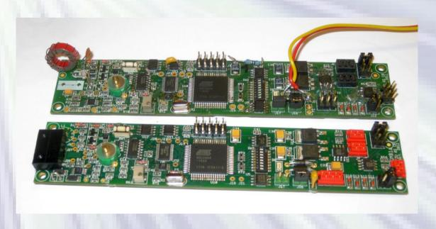
In 2013 we are developing 3 versions of QMB1 with 1.6 ns, 3.5 ns and long pulse 30 ns. Long pulse version is coming with external toroidal inductor.
