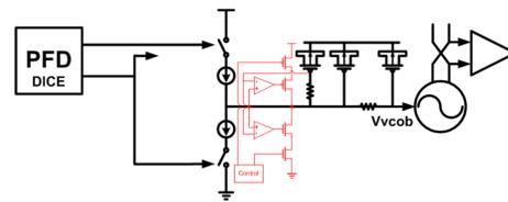
Fig.8 Compensation Solution for SET at the PLL CP output
