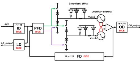
Fig.2 12.5 MHz-500 MHz Radiation-Hardened-By-Design Phased-Locked Loop
