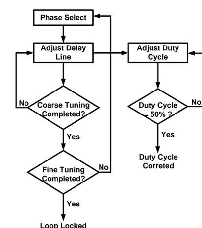
Fig.11 DLL operation procedure
