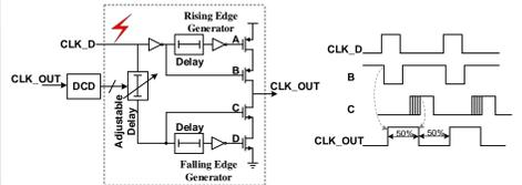
Fig.15 Radiation-hardened duty cycle corrector
