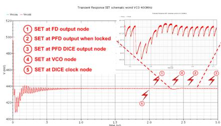
Fig.7 VCO control voltage under single event transient effect (PLL is locked)
