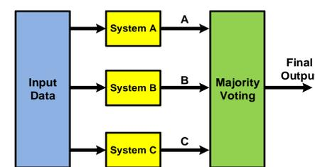
Fig.12 Radiation hardened-triple modular redundancy (TMR)
