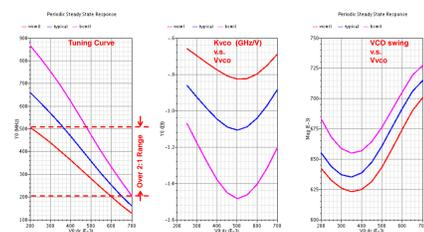
Fig.6 VCO tuning ranges, conversion gain and output amplitude
