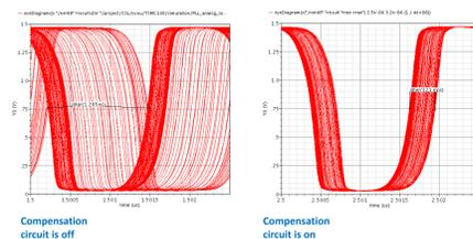
Fig.10 Output clock jitter comparison for PLL w/o V<sub>ctr</sub> compensation circuit
