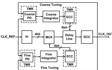
Fig.3 267 MHz Radiation-Hardened Delayed-Locked Loop
