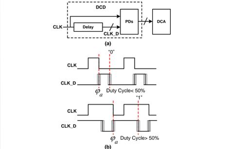
Fig.14 (a) Duty cycle detection circuit (b) Duty cycle detection principle
