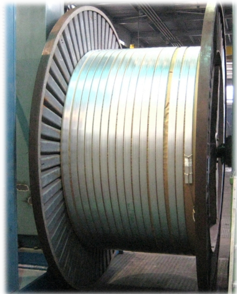
Spool (3 m diameter) with co-extruded conductor
