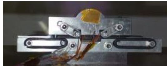
4 points bending test on plates
