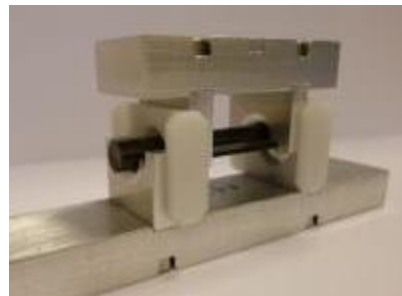
4 points bending test on rods
