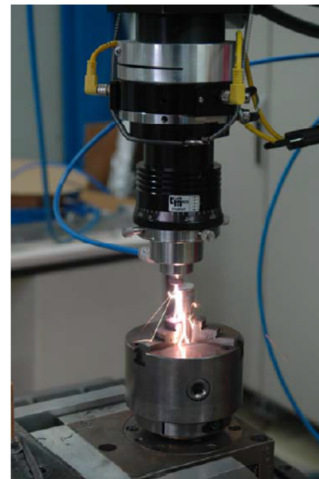
Nd: YAG laser (0.01mm, 1J, 35 W, 610mm/min)
