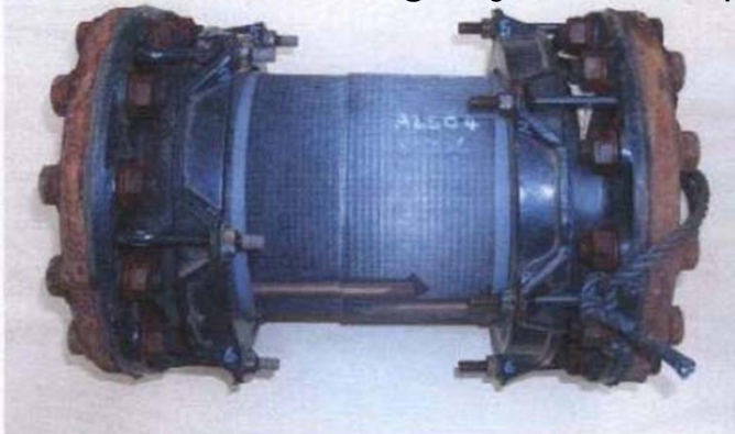
Successful Burst Testing of joined composite
