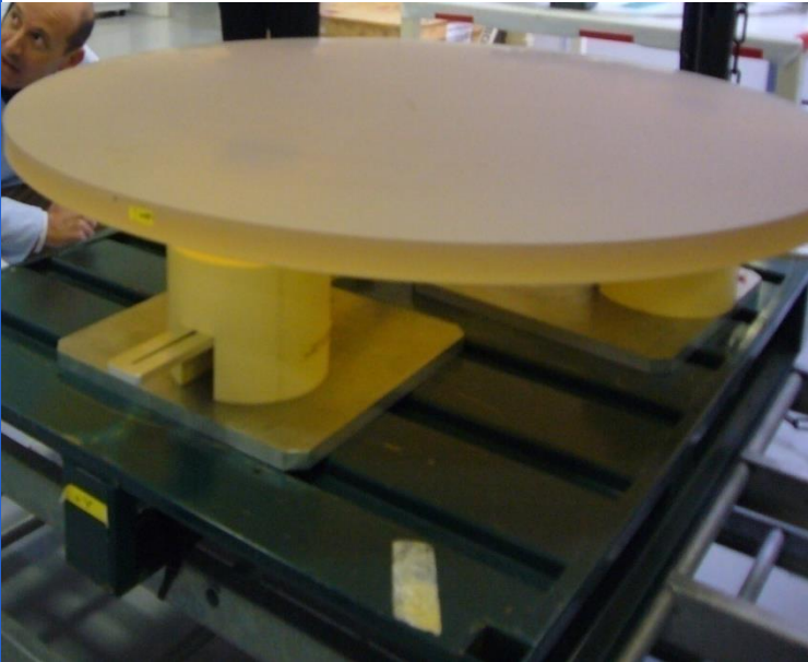
1.1m Zerodur shell manufactured at SAGEM
