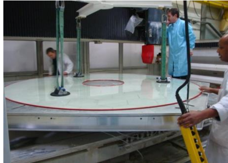
2.6m glass shell, 2 mm thick at SAGEM
