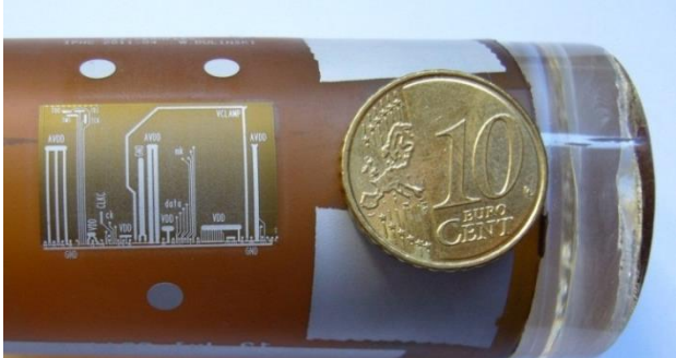
Solid state 50um silicon flexible sensor wrapped over cylindrical shape (R=20 mm)
