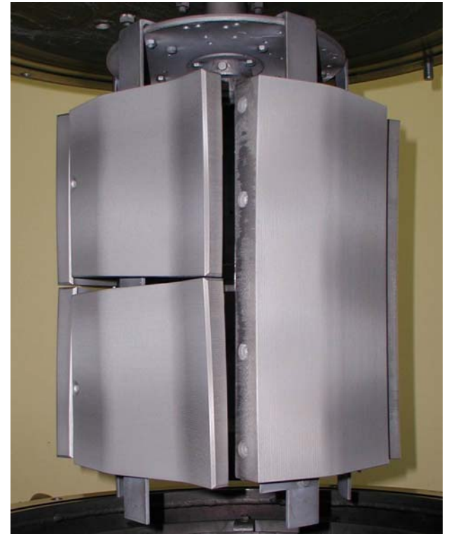
G 6 and G7 divertor tiles coated with 20-25 \mu\text{m} W in series production
