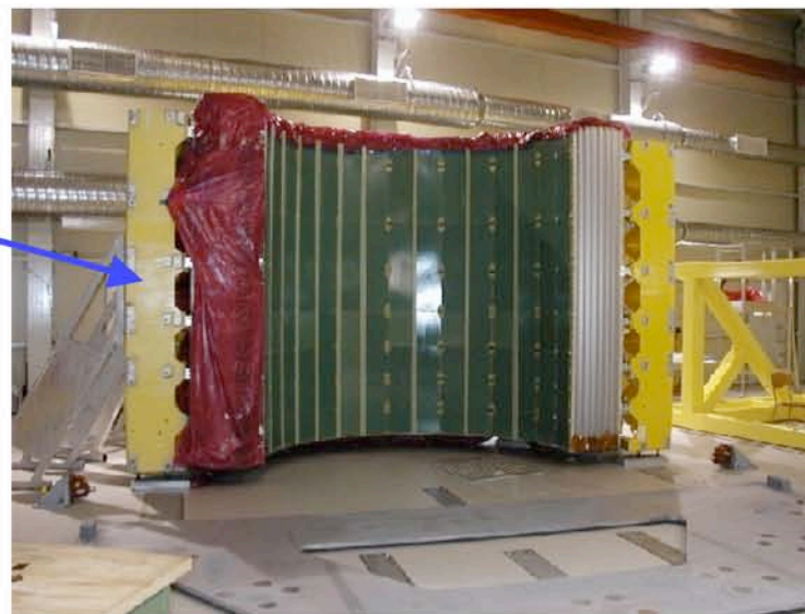
LAr EM barrel assembly in the vertical position
