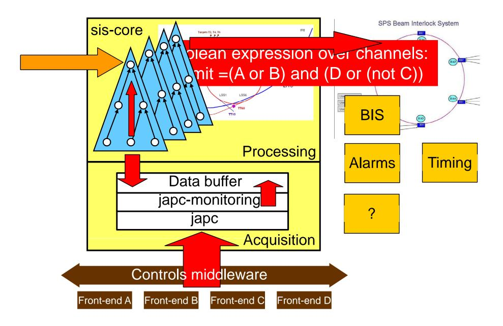
The interlocks are organized in a tree structure. The top level signals are the summary states that are 'exported' to BIC and timing system
