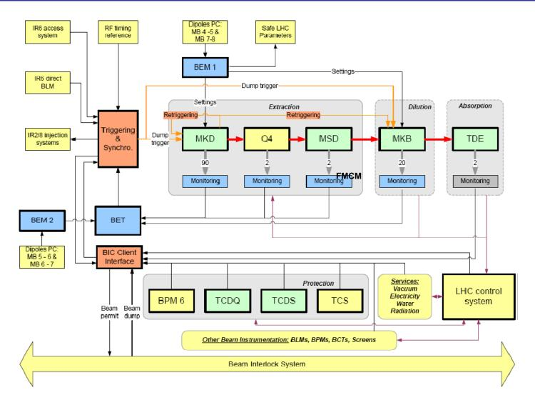
Interfaces: triggering, synchronisation, energy tracking, arming, BIS, injection BIS
