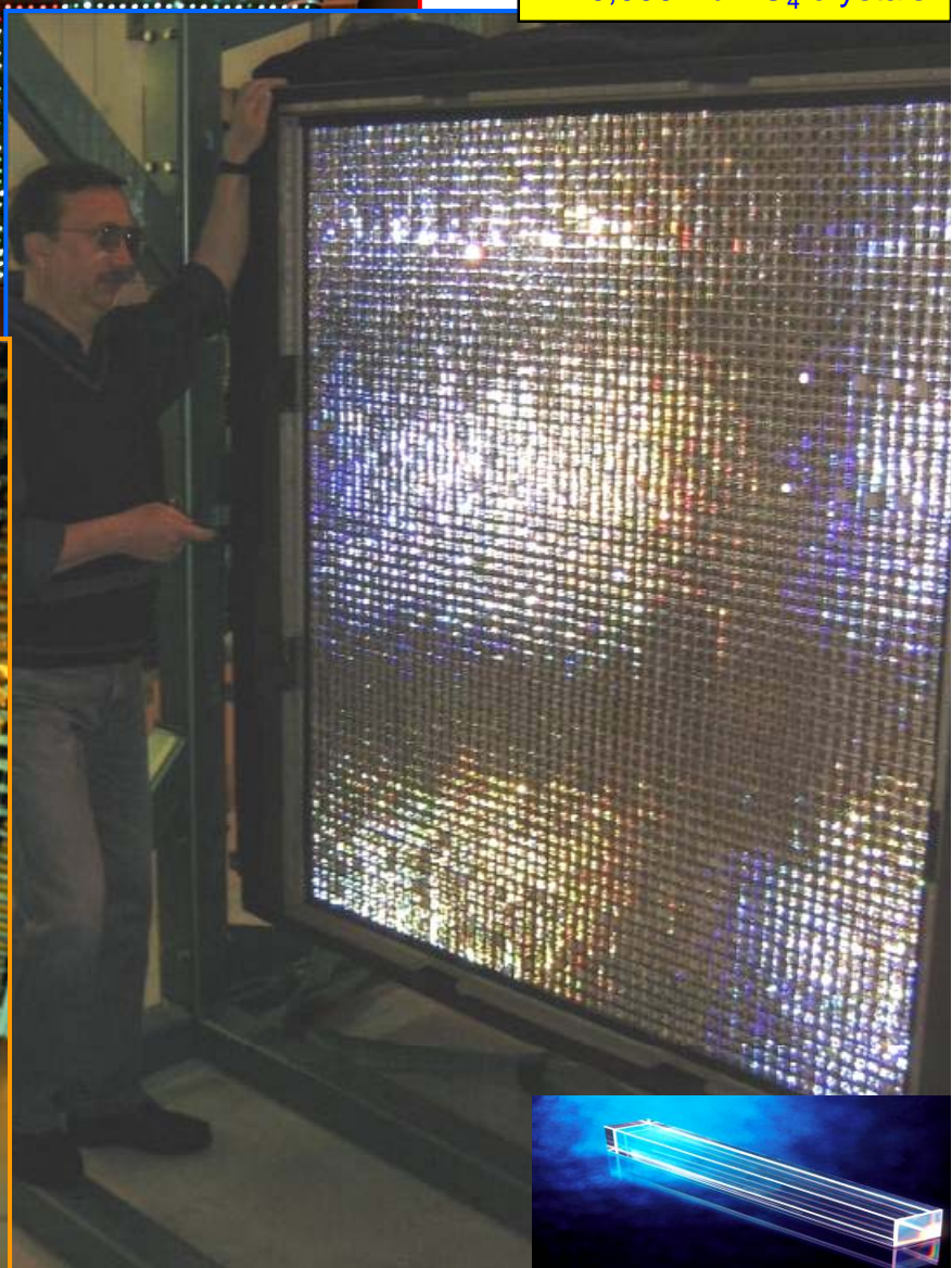
PHOS module ~ 20,000 PbWO 4 crystals
