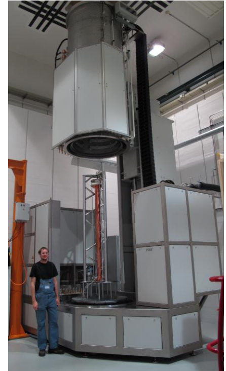
Vacuum brazing furnace installed and operative
