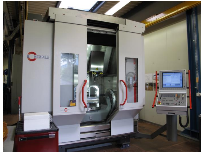
5 axes machine for BOC production (installed and operational)
