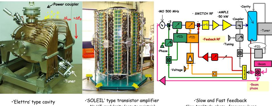
• Elettra Type cavity •3 different tuning knobs Temperature (30÷60 C°, ±0.05 C°) •Mechanical length adjustment ∆l •Tuner on the equator
