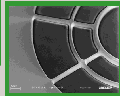
Tungsten - thickness. 100 \mu m Bars : 100 \mu m
