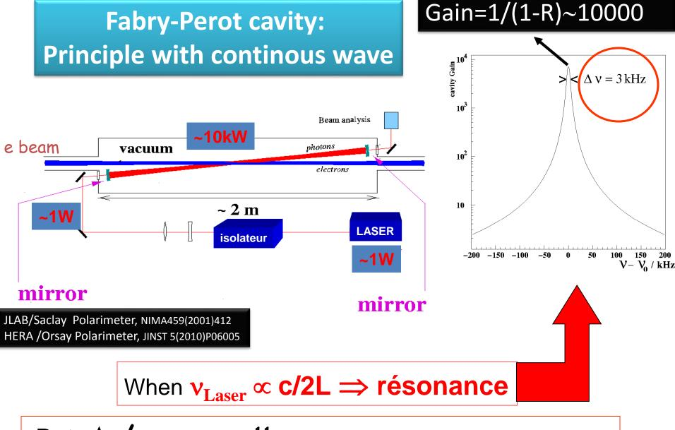
•But:  $\Delta v / v_{\text{Laser}} = 10^{-11} \implies$  STRONG & ROBUST laser/cavity feedback needed...
