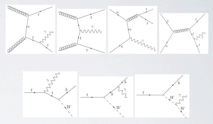
Top production and decay diagrams with  $\boldsymbol{\gamma}$  in the final state
