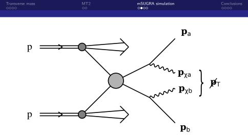
(2) Diagram of a generic process involving two invisible particles in the final state
