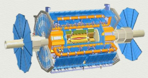
ATLAS - Some cuts in the electromagnetic calorimeter are applied (central barrel  $|\eta| < 1.475$ , and end-cap regions on either end of the detector  $1.375 < |\eta| < 2.5$ , for the outer wheel and  $2.5 < |\eta| < 3.2$  for the inner wheel) in order to have more efficiency in the analysis
