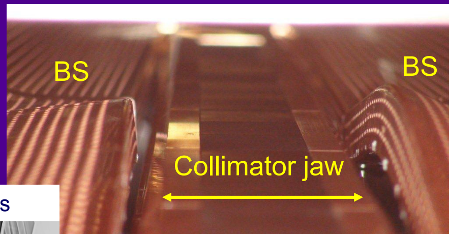
Damaged beam screen (BS) in a collimator
