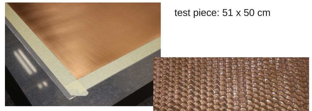
roughing the surface => remove CuO + surface treatment with acetone
