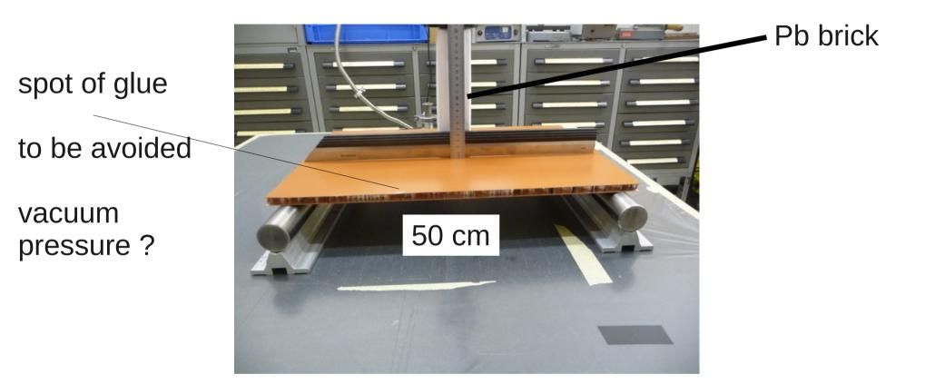
bowing of 0.85 mm @ 11.34 kg stable over 3 days reversible => ? thicker panels on exterior of quadruplet ?  $\sim D^3$
