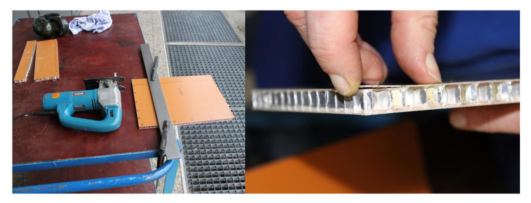
jig-saw is rocking and shaking headset needed => FORCE the cutting of the honeycomb bars is noticed the FR4 delaminates only at the edges the glue joint is stable in the interior
