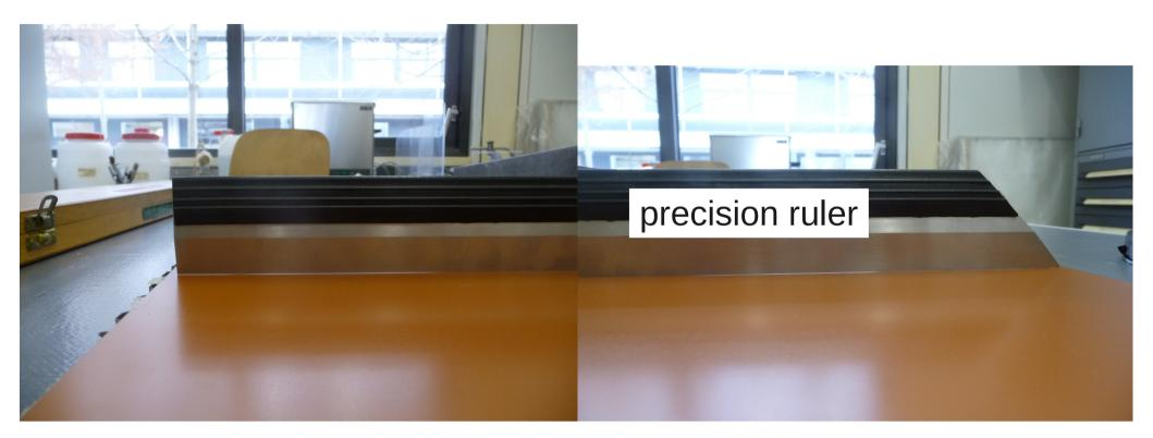
accuracy of planarity at some points only 0.1 mm mostly better than 0.05 mm 3 measurement positions each in both directions
