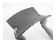
konvex - konkav deformation in X – Y direction
