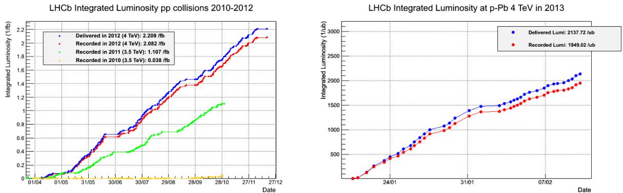
Figure 1: LHC delivered luminosity at the LHCb interaction point and LHCb recorded luminosity for 2012 (left), and 2013 (right).
