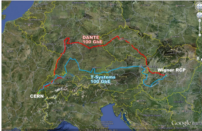
Figure 6: Networking between CERN and Wigner data centres: 2 independent 100 Gb/s lines
