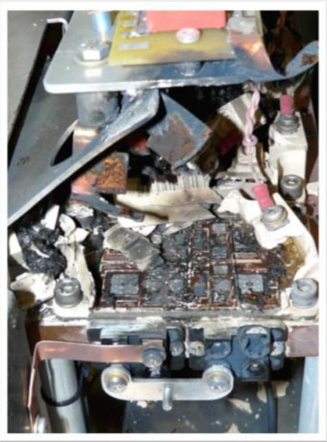
3Hz Booster dipole power supplies : upgrade IGBT class (400A to 600A) but was not sufficient. The number of operating cycles is larger than expected. A redesign of these units is progressing.
