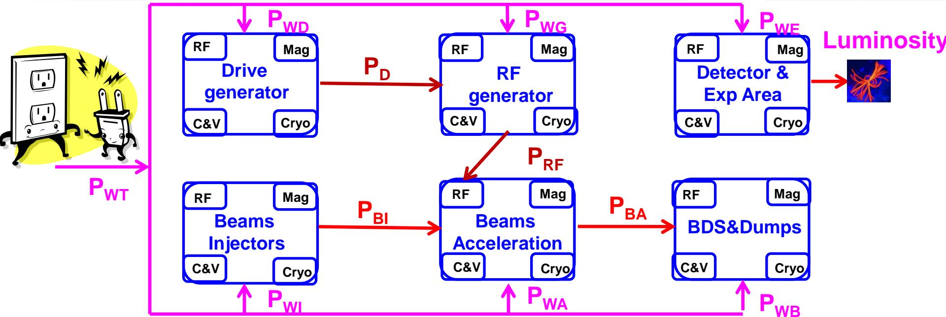
Figure of merit:  $\eta_L = \text{Luminosity}/P_{WT}$
