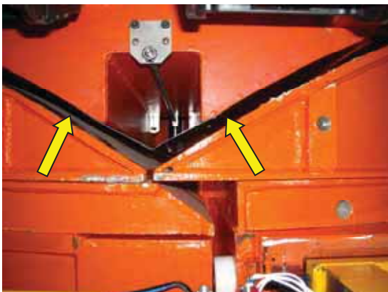
(The wooden shims can be removed with the remnant magnetic field)
