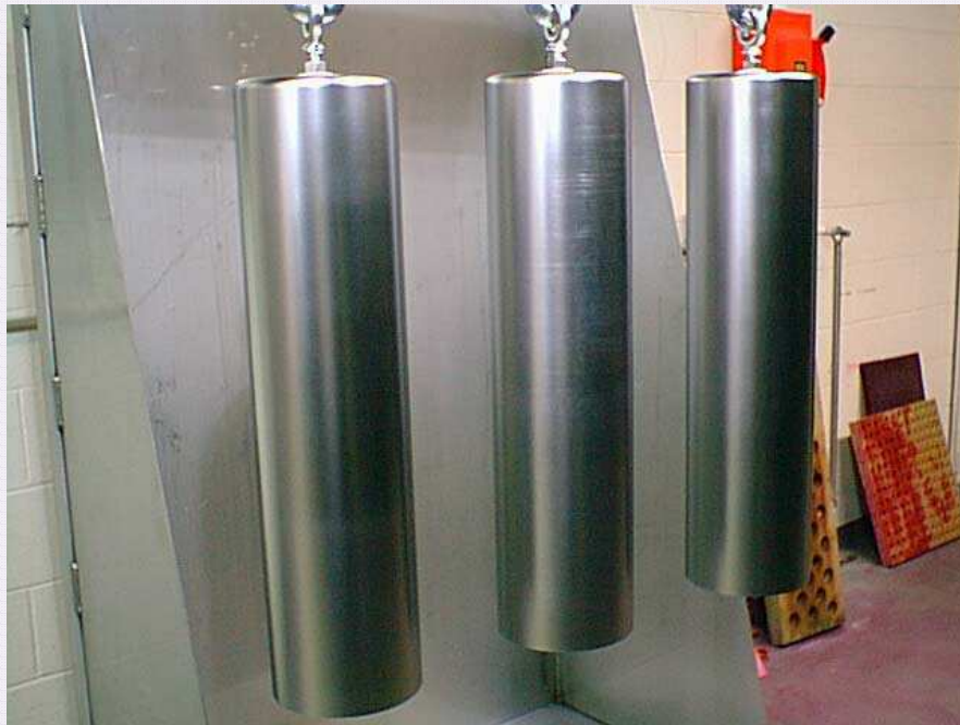
Nb-Ti Billets ( \Phi = 30 cm)
