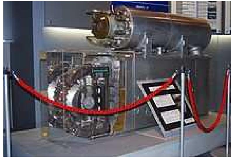
Superconducting magnet and a liquid helium tank on top of it
