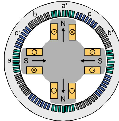
Superconducting synchronous machine
