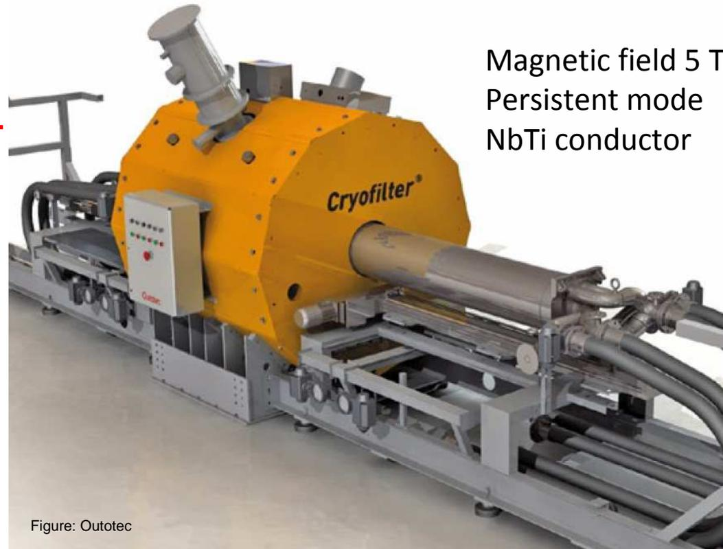
Industry solutions are offered for magnetic separation with LTS
