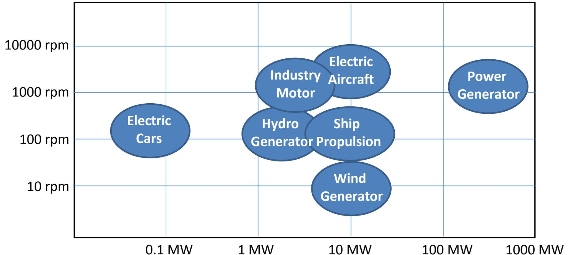
There are many potential applications for HTS rotating machines that differ very much in rating, torque and speed.
