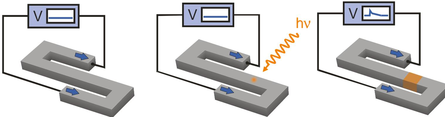
Single-photon sensitivity from visible to infrared spectrum, e.g. ultrafast spectroscopy
