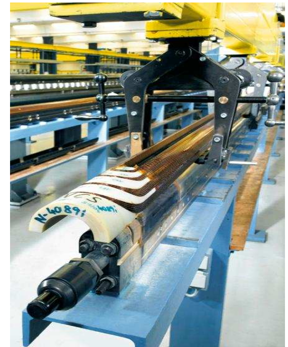
Layerjumps on LHC main dipole winding package
