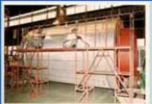
Superconducting solenoid coil was being made at Hitachi company.
