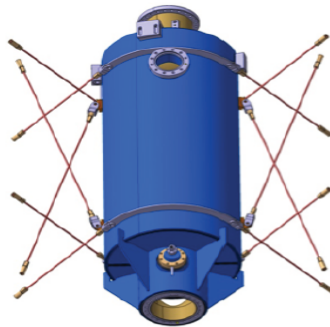
Figure 4.120: Helium vessel with hanging rod
