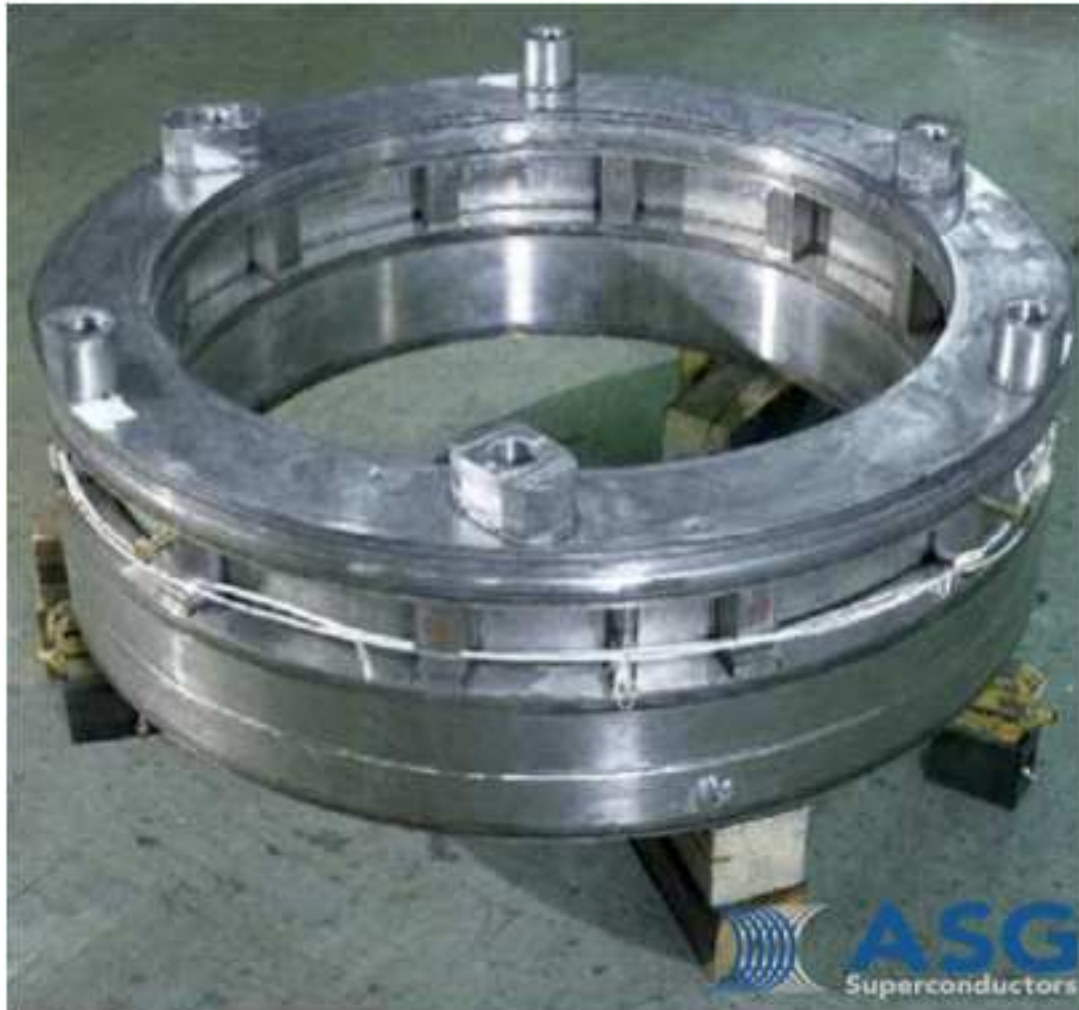
Lower module of welded mechanical structure
