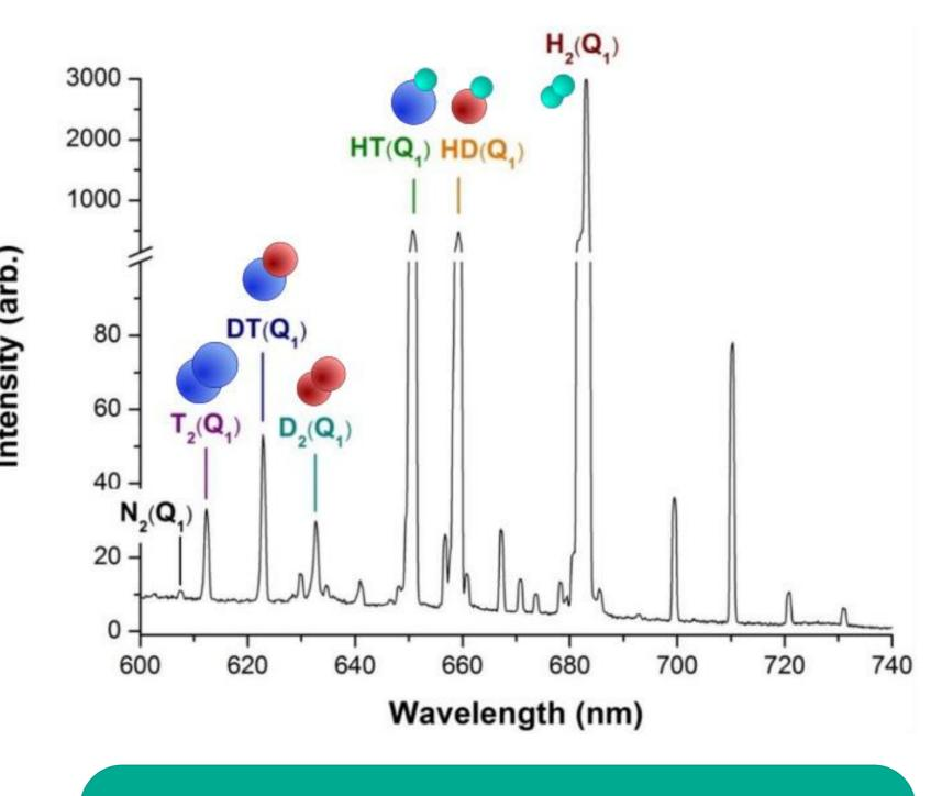
Quantitative analysis of gas sample composition based on Raman line intensities
