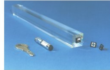
A full size (23cm long) lead tungstate crystal with a mounted APD
