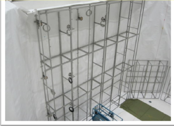
PMT supporting structure + tyvek+PMT
