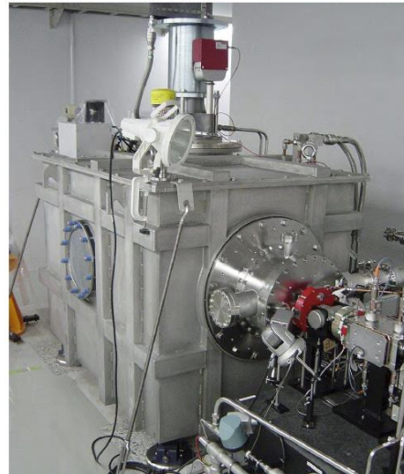
500 kV Electron Gun
