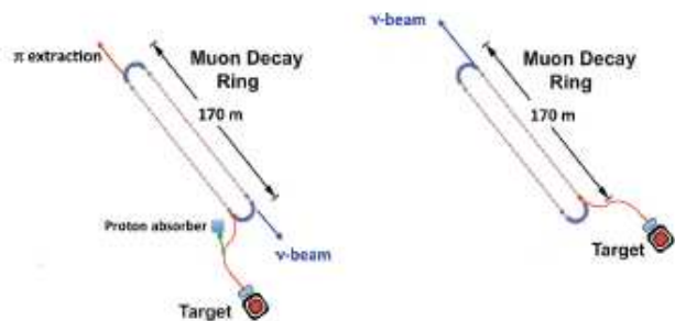
Figure 9: The \mu STORM facility, with a Decay Ring having 150 m straights and 25 m, 180° arcs. The left figure shows a possible CERN layout where injection of pions produced from the full 10 \mu s spill of 100 GeV protons from the SPS would correspond to \sim 7 turns of the muon beam in the storage ring. The FNAL option, to the right, injects pions produced during only 1 \mu s 60 GeV proton extraction from the Main Ring.
