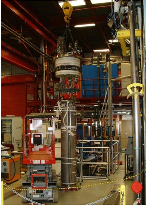
MBHSP01 mechanical and electrical connection to the Top Heat in IB1 (FNAL MTF)
