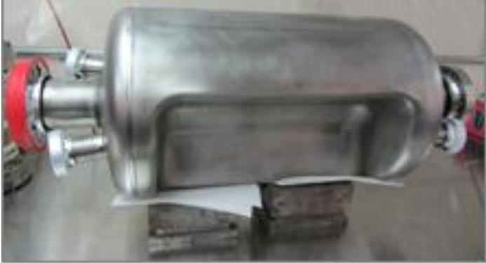
RF-Dipole Nb prototype [ODU-SLAC]
