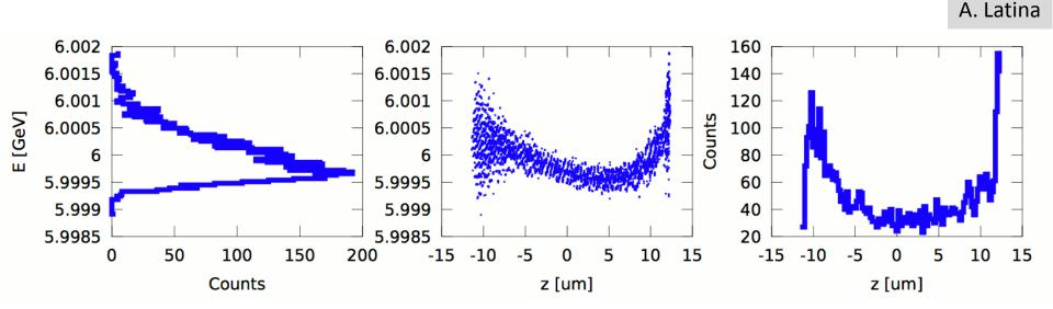
Structure with a/ $\lambda$ =0.14 and G=67.5MV/m used  $\sigma_z$  = 7.96 µm,  $\sigma_E$  = 0.0071%,  $\sigma_{E,slice}$  = 0.0027% (for comparison Swiss FEL target at undulator  $\sigma_{E,slice}$  = 0.006%)
