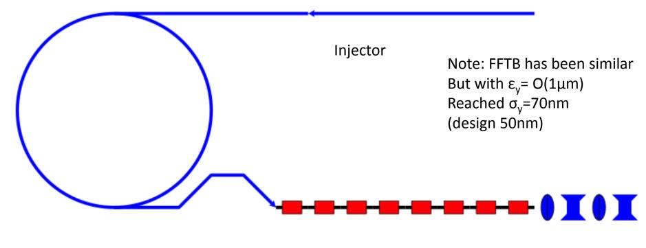
Low emittance ring, e.g. CLIC damping ring, 3<sup>rd</sup> generation light source, damping ring test facility Main linac with bunch compressor Powered with drive beam or X-band klystrons
