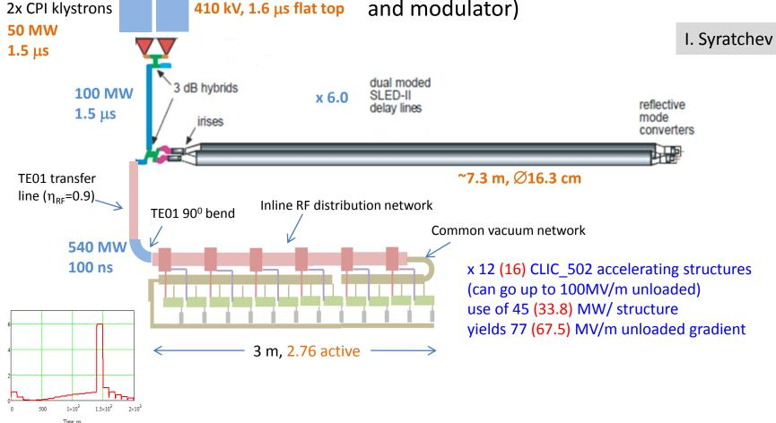
This unit should provide ~213 (248) MeV acceleration beam loading. Need 27 (23) RF units. Future CLIC klystrons would save O(20%)
