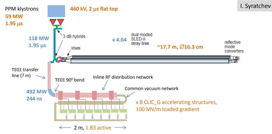
This unit should provide ~221 MeV acceleration without beam loading. The adopted components (klystron, modulator, RF network and structures), are expected to operate at the edge of demonstrated performance. Some of them (like 2-pack solid state modulator) need industrialization efforts.
