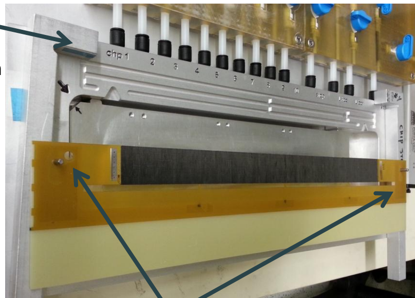
Cable reference holes for assembly
