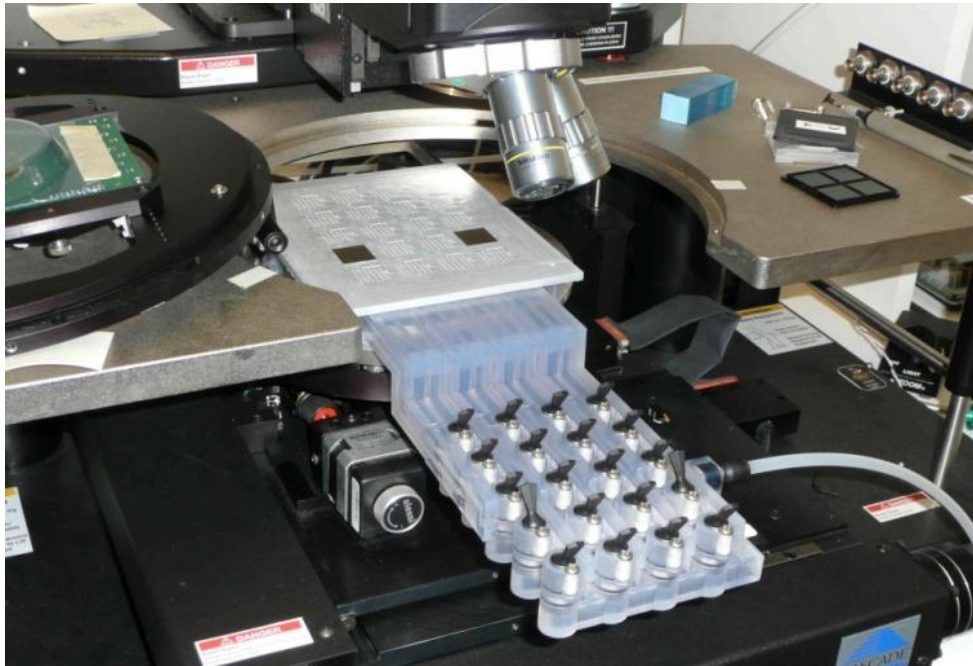
Vacuum chuck for testing 20 thin sensors (50 \mu\text{m} ) Testing up to 18 sensors per batch Manual alignment
