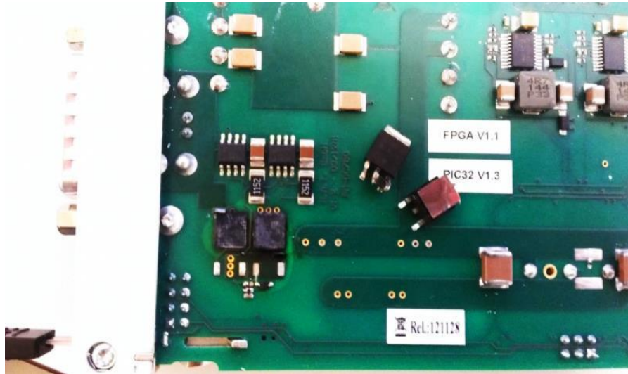
PM PCB bottom layer after failure
