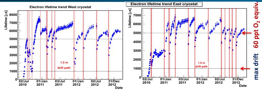
LAr continuously filtered,  $e^-$  life-time measured by charge attenuation study on cosmic  $\mu$  tracks.
