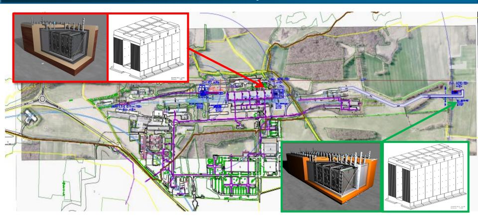
100 GeV primary proton beam fast extracted from SPS, ~ 110 m decay pipe, beam dump followed by  $\mu$  stations. Interchangeable  $\nu$  and  $\bar{\nu}$  focusing. Near detector (T150 - to be built) at 460 m, far detector (ICARUS-T600 - to be moved to CERN) at 1600 m, both coupled to magnetic spectrometers.
