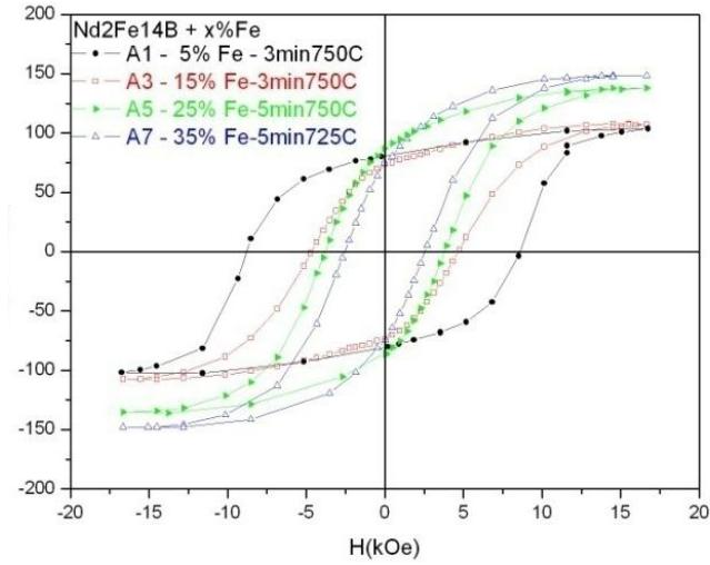
Nd-Fe(Ti/Zr)-B: increases the energy product from 150 kJ/m<sup>3</sup> to 250 kJ/m<sup>3</sup>
