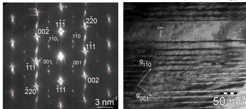
SAED pattern of a specimen region oriented along  $\mathbf{B} = [110]$ ; tetragonal system:  $a=b=3.78$  Å,  $c=3.29$  Å,  $c/a=0.87$ ; twinning plane  $(-111)$ ; red spots correspond to the matrix lattice; green spots correspond to the twin stripes. TEM image of the twinned region
