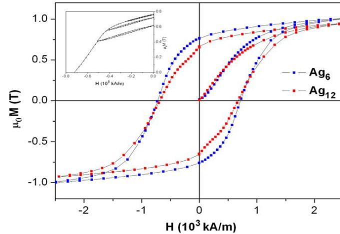
$\text{Fe}_{48}\text{Pt}_{28}\text{Ag}_6\text{B}_{18}$  as cast -  $(\text{BH})_{\max}=87 \text{ kJ/m}^3$
