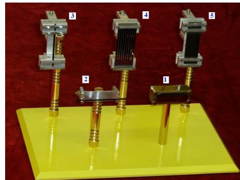
the Principle of a bend of a strip-type crystal (the device 3). The necessary cross-section bend is created by a longitudinal bend of a plate due to anisotropy of a crystal.
