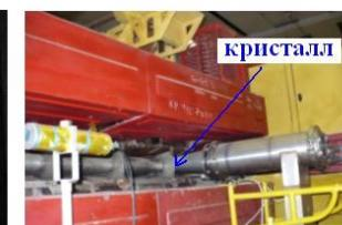
the extraction of a beam from U-70 ring by crystals 1 and 2 in a direction of beam lines N2 and N4.
