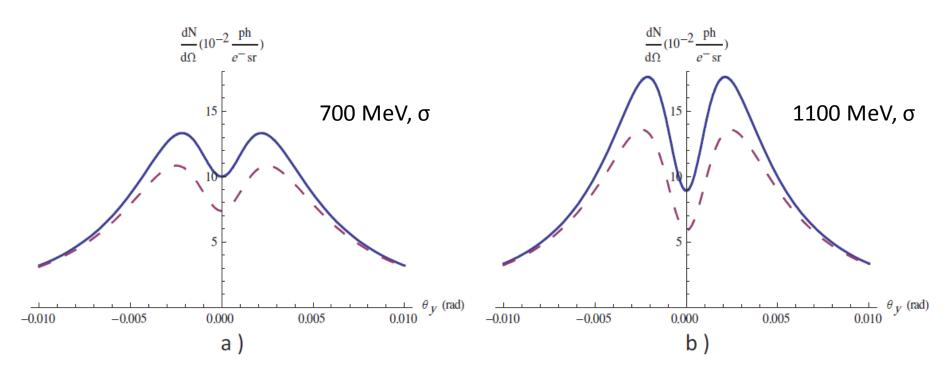
Increase of the PXR intensity for (111) reflection in crystal Si with thickness  $L = 500 \, \mu m$ ,  $L_{abs} = 392.6 \, \mu m$ ;  $\hbar \omega_B = 14.4 \, \text{keV}$ ,  $\theta_B = 7.89^\circ$ ,  $\beta = 0.962$ ,  $\sigma$ -polarization (solid curves correspond to the dynamical theory, dashed lines correspond to the kinematical one): (a)  $E = 700 \, \text{MeV}$ , (b)  $E = 1100 \, \text{MeV}$ .
