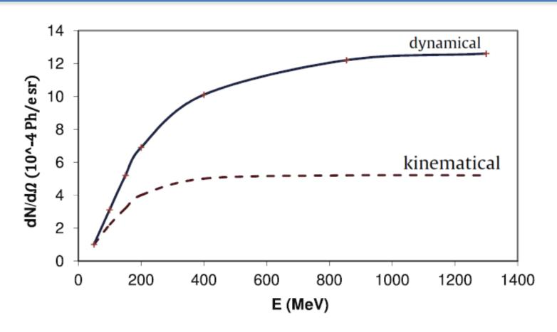
Dependence of the maximal PXR intensity on the electron energy for (220) reflection in crystal Si with thickness  $L=124~\mu m,\,L_{abs}=19.56~\mu m,\,L_R=9.4~cm$   $\hbar\omega_B=5.166~keV,\,\theta_B=38.7^\circ,\,\,\beta=0.219$
