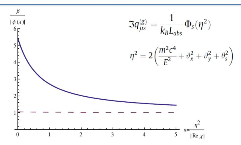
Characteristic behavior of  $\beta/\Phi_{\sigma}(x)$  (solid line) and  $\beta/\Phi_{\pi}(x)$  (dashed line) for the reflection (220) in crystal Si. The radiation parameters are following:  $\hbar\omega_{B}=5.166$  keV,  $\theta_{B}=38.7^{\circ},~\beta=0.219$ .
