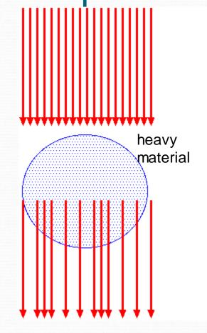
absorption (amplitude attenuation)
