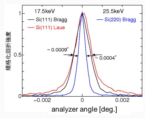
Using a 3<sup>rd</sup> analyzer crystal in the (+,-,+) arrangement, the whole of a PXR beam can be diffracted with a narrow angular width despite the cone-beam. (pseudo-plane wave)
