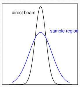
small-angle scattering: reduction of the peak height (or peak broadening) of the curve
