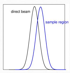
refraction: shift of the center of the curve
