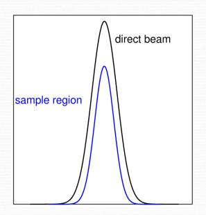
absorption: reduction of the area of the curve
