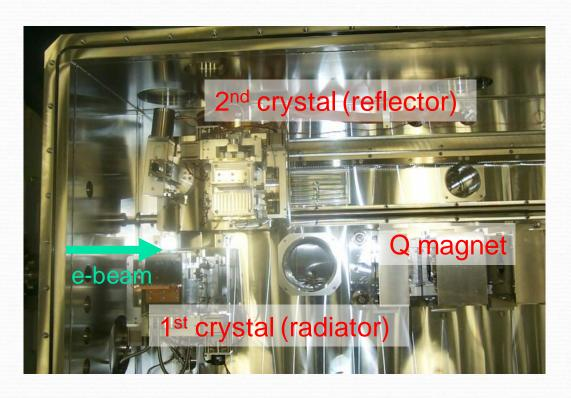
PXR radiator: 0.2mm thick Si perfect crystal wafer reflector: 5mm thick Si perfect crystal plate crystal plane:
