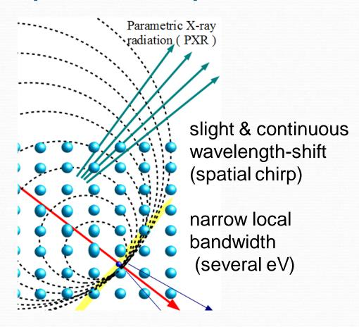
Wave front of PXR is different from both plane wave and spherical wave.
