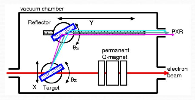
To actualize an X-ray source based on PXR, a double crystal system was proposed and developed.
