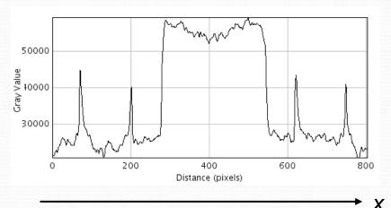
the contrast is sensitive to the styrene-foam region independently of the density and the shape of the sample.
