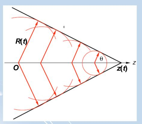
Cherenkov Radiation is generated whenever the charged particle velocity is larger than the phase velocity of light
