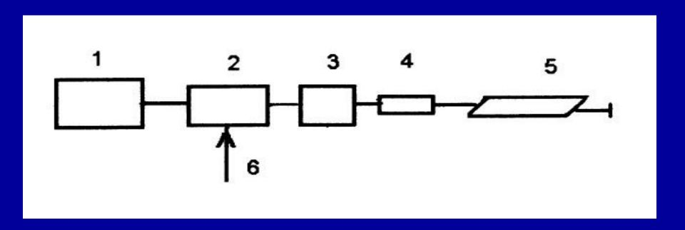
To the control input of the PWM converter 2 is given the modulating frequency 6. Small resistive ballast 4 serves to overload protect the magnetron 5. Multiplier 3 capacitors are selected so, that the high output voltage which supplied to the magnetron 5, comprises a constant and variable components and repeats the shape of the curve modulating signal 6.
